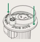
1. Align wide tab on flange cover with wide space on case and press flange cover onto case.
