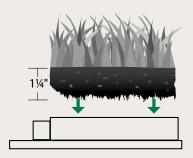
3. Using a standard golf-hole cutter, cut a sod plug. Place small slice in the center of the plug to accept the pull up tab. Install sod into cup and press firmly into place.
