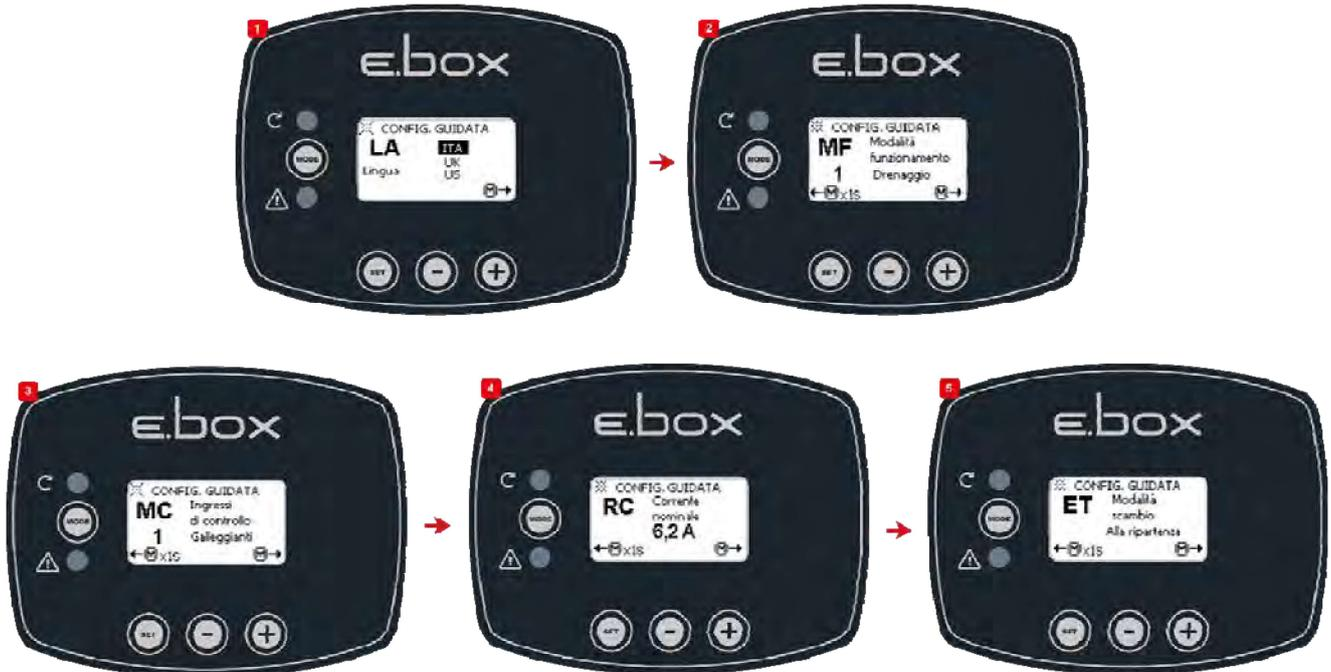
Figure 36: Configuration of Drainage floats or level probes
