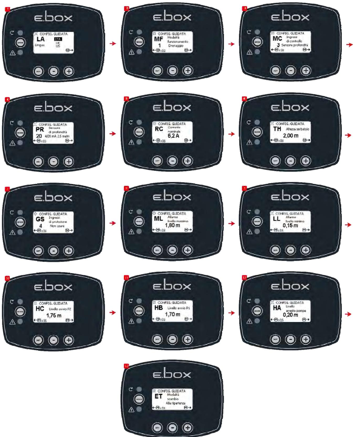
Figure 38: Configuration with only a depth sensor
