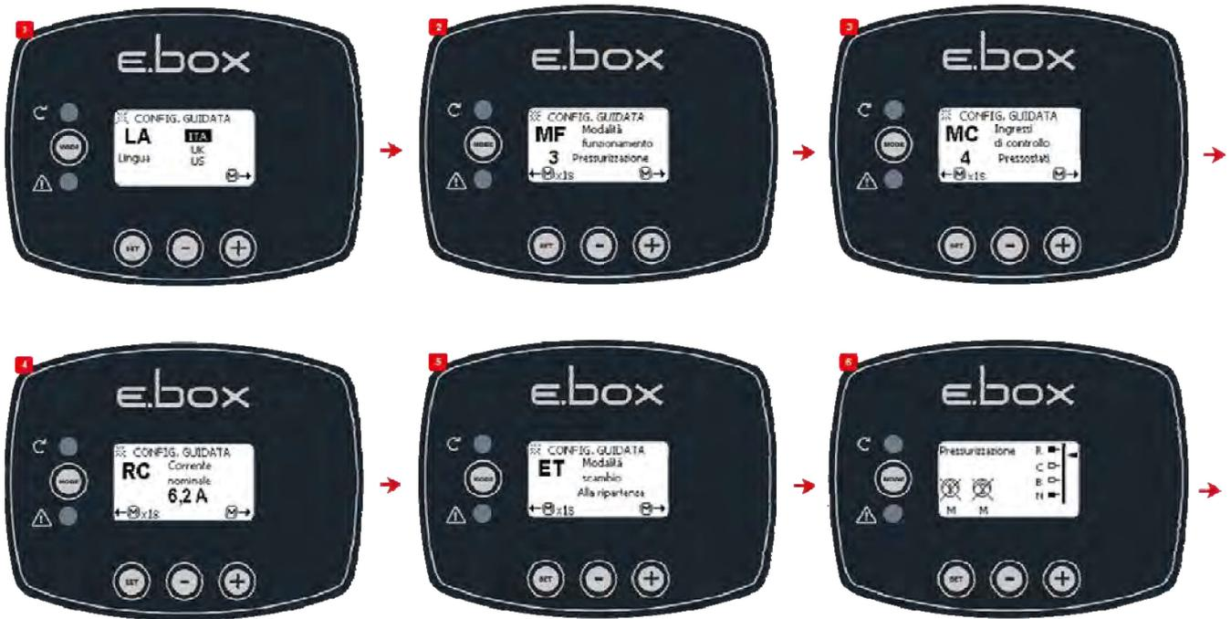
Figure 13: Configuration with pressure switches
