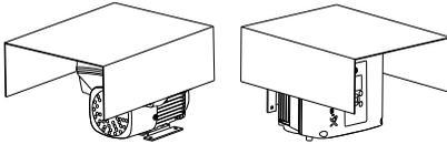
Fig. 8 Examples of covers (not supplied by Grundfos)
