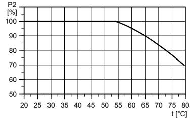
Fig. 13 Derating in relation to the ambient temperature
