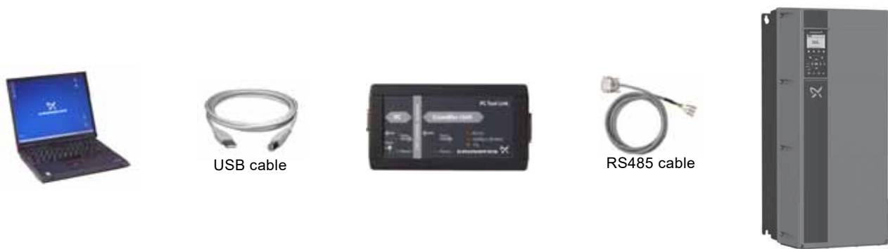
Fig. 8 Connecting the computer to CUE using PC Tool Link (USB)
