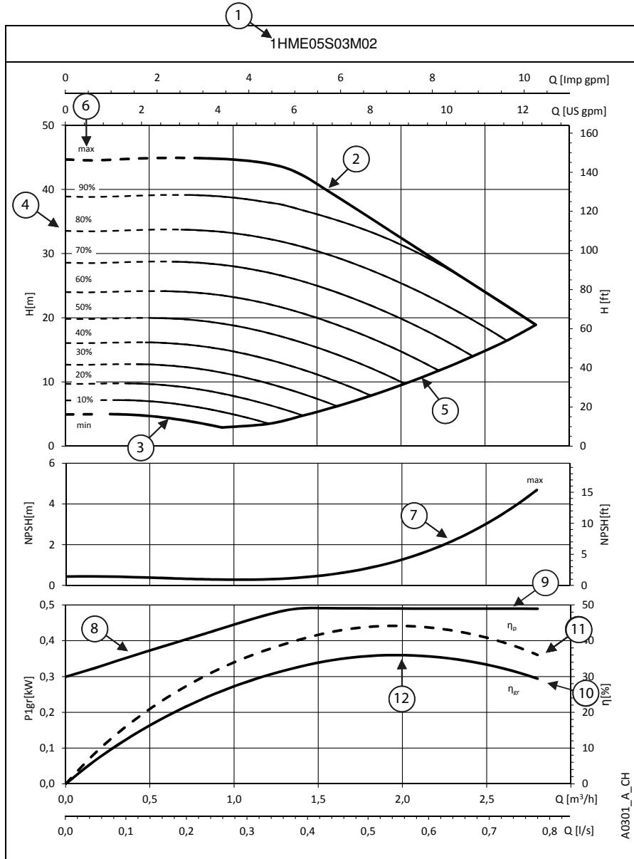
⑥ The **part load percentage** is calculated depending on maximum speed (*max*, 100%) and minimum speed (*min*, equal to 0%, which is the minimum part load step, below it the drive stays powered up but cannot work).
