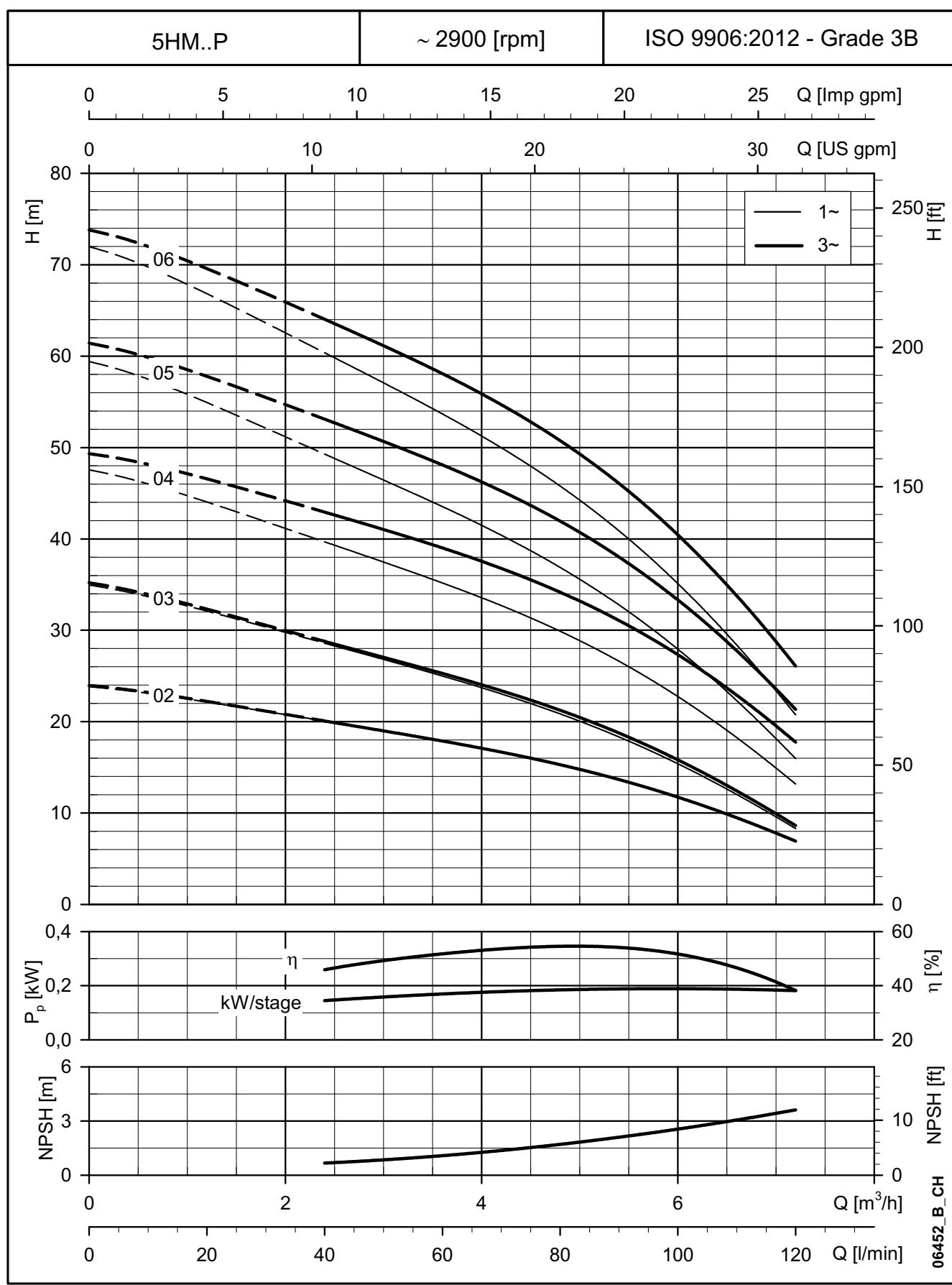
These performances are valid for liquids with density  $\rho = 1 \text{ Kg/dm}^3$  and kinematic viscosity  $v = 1 \text{ mm}^2/\text{sec}$ .
