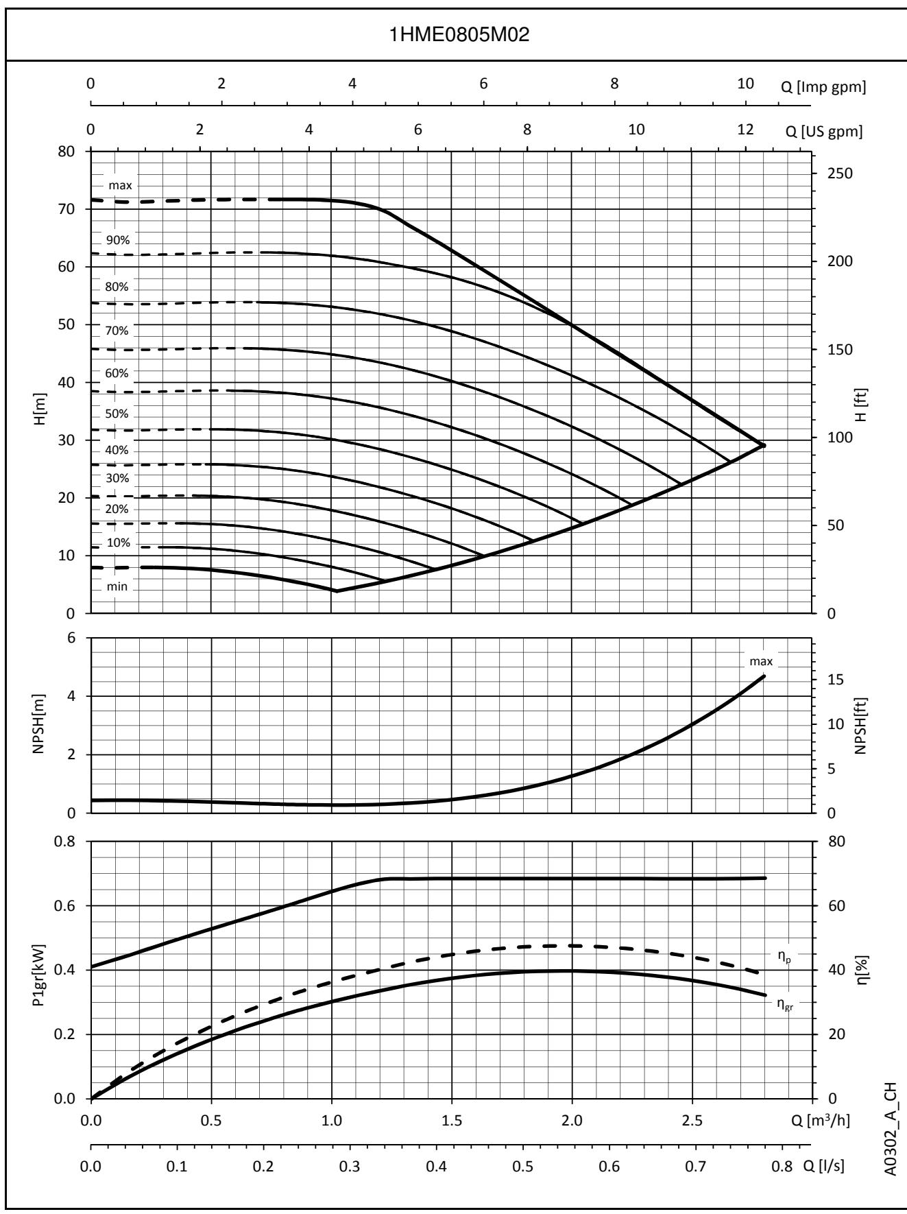
The performances are valid for liquid with density  $\rho = 1 \text{ Kg/dm}^3$  and kinematic viscosity  $\nu = 1 \text{ mm}^2/\text{sec}$ .
