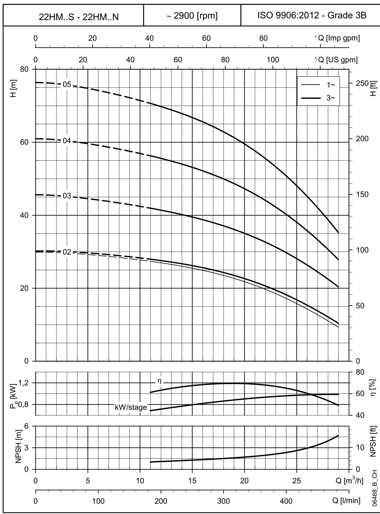
These performances are valid for liquids with density  $\rho = 1$  Kg/dm<sup>3</sup> and kinematic viscosity  $\nu = 1$  mm<sup>2</sup>/sec.
