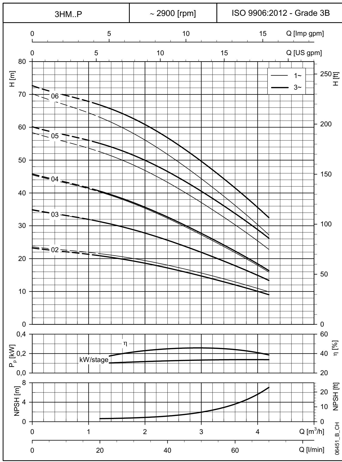
These performances are valid for liquids with density  $\rho = 1 \text{ Kg/dm}^3$  and kinematic viscosity  $\nu = 1 \text{ mm}^2/\text{sec}$ .
