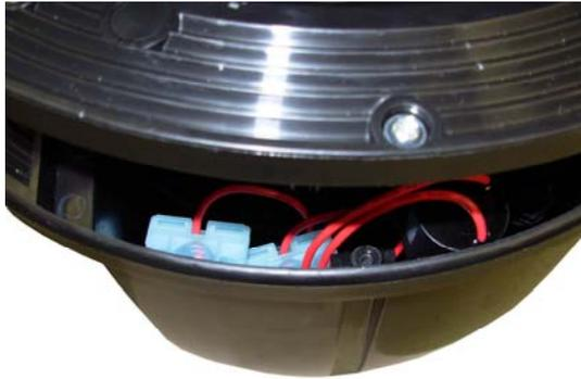
Put back the cables into the cable compartment and close the cover.
