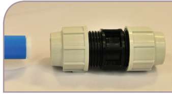
Insert liner into pipe (metric 20mm-63mm only) and slacken nut until half the thread is visible.
