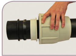
Draw the nut, collars, and 'O' ring over the end of the pipe to a distance of approx. 250mm (put the white split ring to one side for later use).
