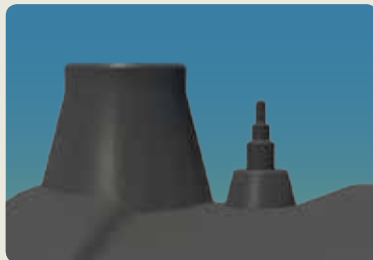
Sample of raised melt indicator after welding
