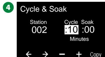
5 Press the + and – keys to set the Soak time (between 1-60 minutes).
