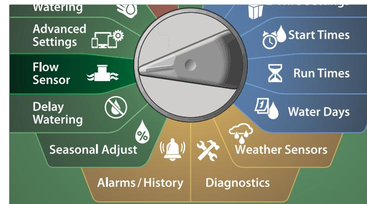
1 At the FLOW SENSOR screen, with Set Flow Rates selected, press Next.
