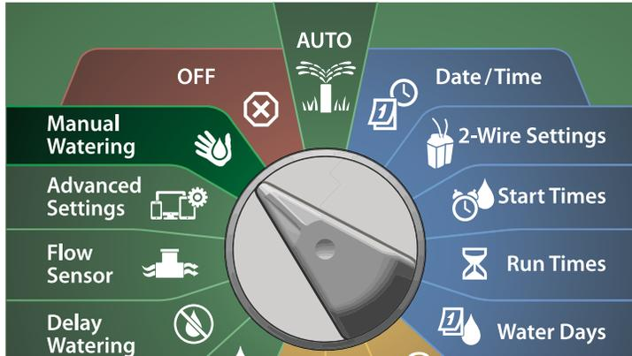
**1** At the Manual Watering screen, press the Down Arrow key to select Test All Stations, then press Next.
