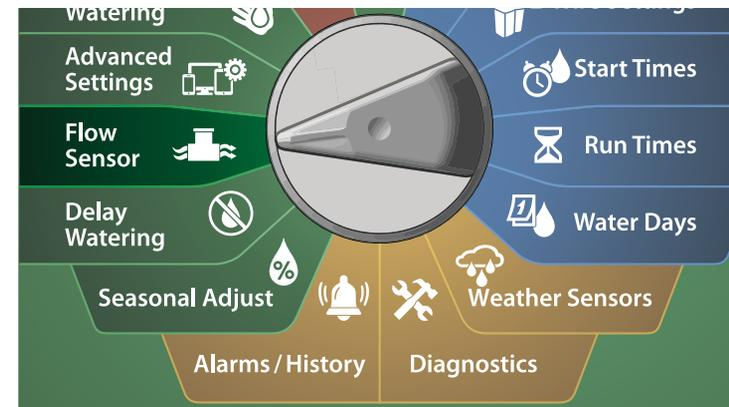
1 At the FLOW SENSOR screen, press the Down Arrow key to select Set Current Flow Reading, then press Next.
