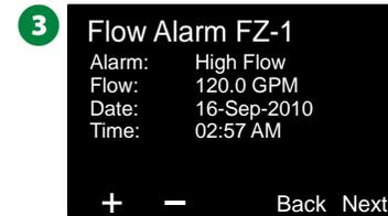
Note each station which has an alarm, then see "Clear Flow Alarms" on page 65 for more details on how to clear flow alarms.
