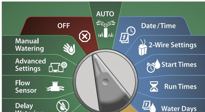
1 At the All Watering Off screen, press the + and – keys to adjust contrast up or down (from 0 to 12).
