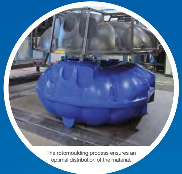
The rotomoulding process ensures an optimal distribution of the material.
