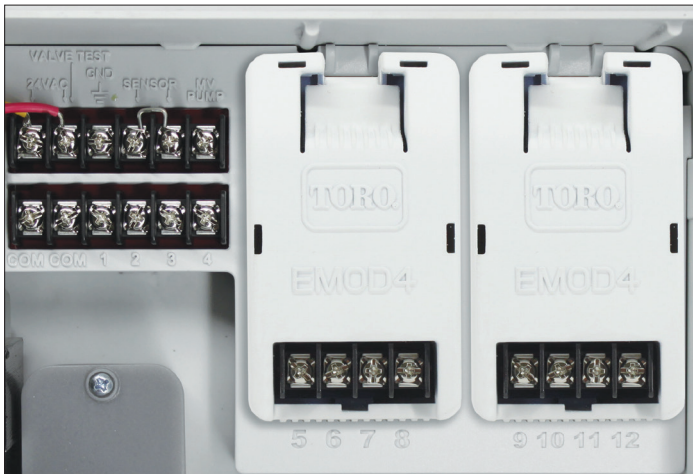
12-station configuration with two four station modules (EMOD-4)
