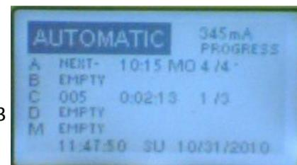
Whilst No. 5 is running, the decoder line current and Master Valve are collectively taking 345mA. This is the summation of all the standby currents of the decoders, the Master Valve and the solenoid attached to decoder 5.
