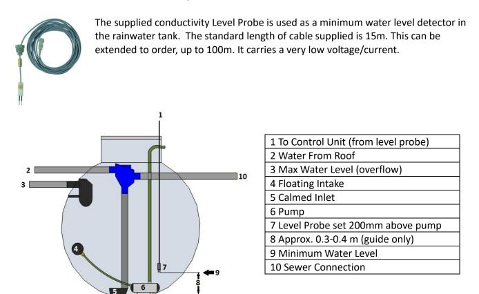
Fix the Level Probe in the tank so that it is suspended approximately 0.3 to 0.4 metres above the bottom, depending on the shape of the tank and position of pump inlet. It should be positioned to ensure there is no risk of cavitation or air entrainment to the pump inlet. If in doubt you MUST consult an approved and qualified plumber. The height of the Level Probe determines the minimum water level of the tank at which the pump will run.
