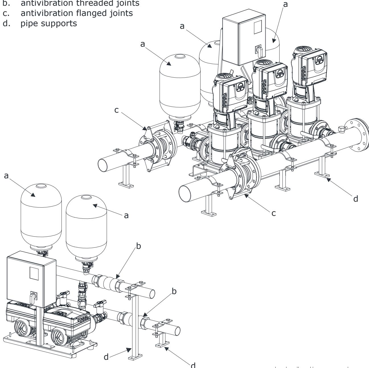
The booster set is connected to pressurised tanks.
