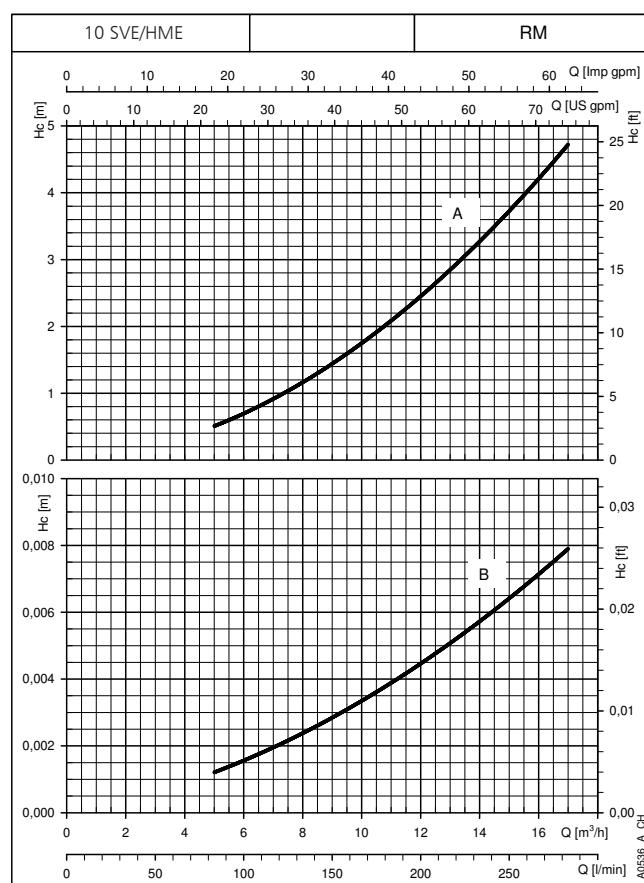
The declared curves are valid for liquids with density  $\rho = 1 \text{ Kg/dm}^3$  and kinematic viscosity  $v = 1 \text{ mm}^2/\text{sec}$ .
