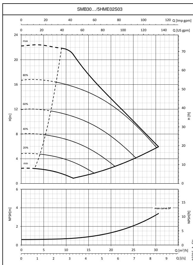
The performance curves do not take into account flow resistance in the valves and piping.
