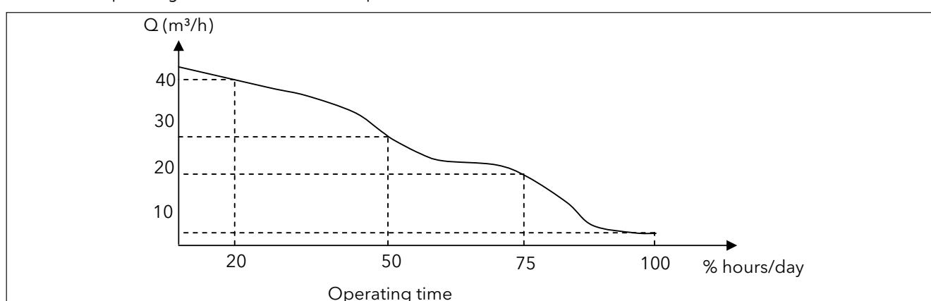
When selecting the booster set the consumption figure of the system must be considered, which is generally supplied by the person who designed the system. For systems where consumption varies continuously and suddenly over time it is advisable to install SMB series booster sets with variable regulation of the electric pump speed.
