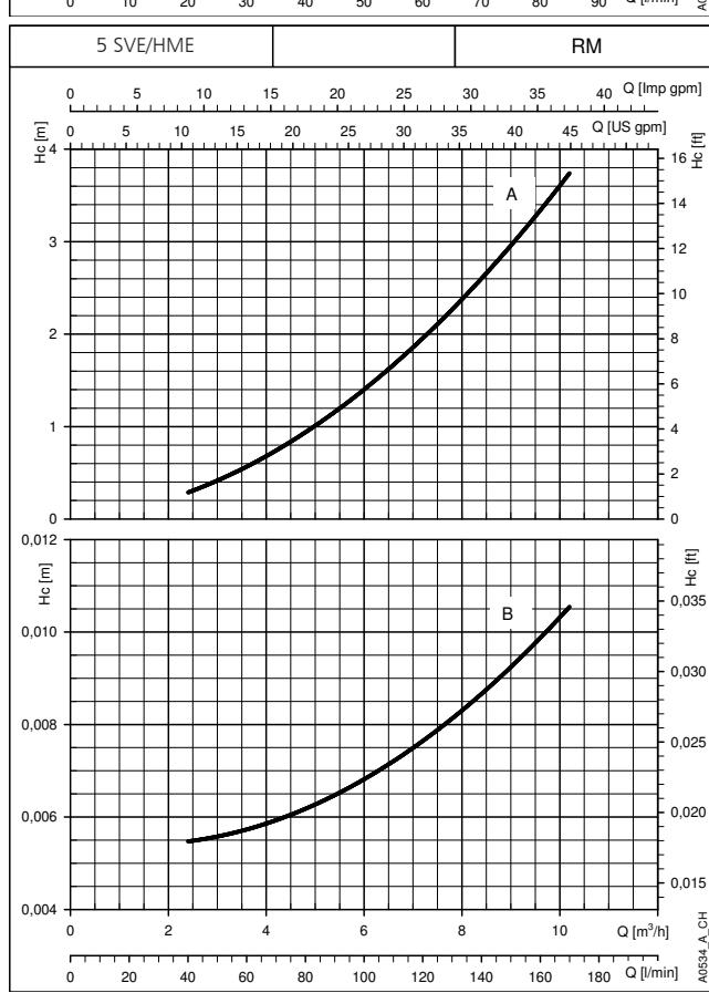
The declared curves are valid for liquids with density  $\rho = 1 \text{ Kg/dm}^3$  and kinematic viscosity  $v = 1 \text{ mm}^2/\text{sec}$ .
