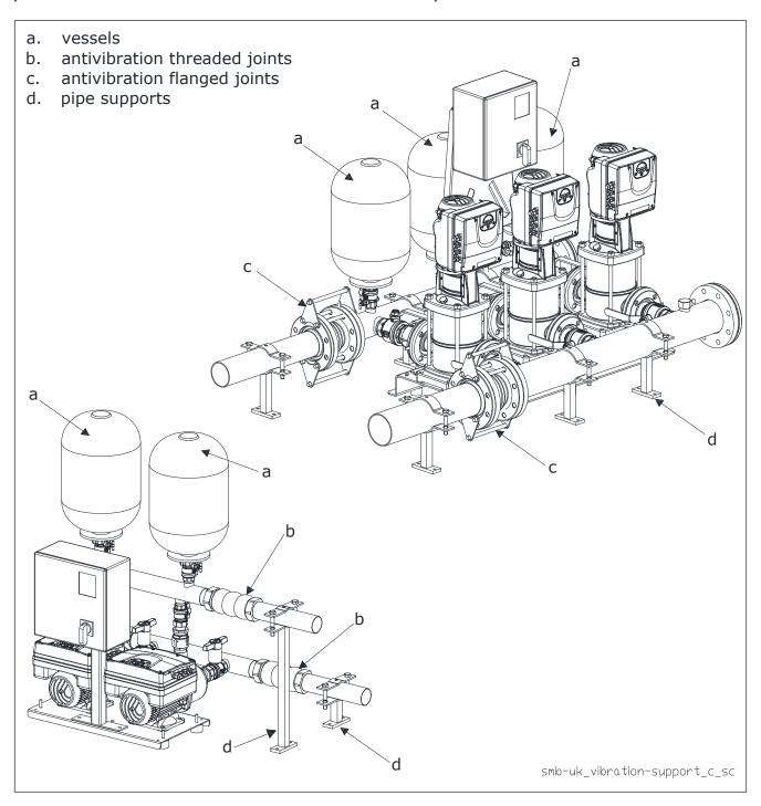
The booster set is connected to pressurised tanks.
