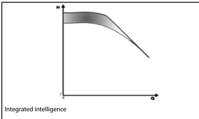
**Adjustment:** This is possible both at constant pressure and according to the characteristic curve of the system, based on the customer's preferences. Another option is according to an external signal or at a preset speed.
