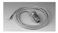
Sensor for detecting the presence of water based on the optoelectronic principle, therefore non-invasive and with no moving parts. The sensor features an electronic contact (on/off) which stops the pump if there is no water in the seal area.
