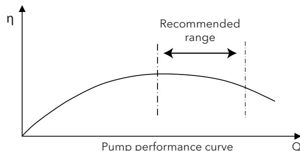
If we make a choice on the characteristic curve of the electric pump, we can see that the optimum working area where the booster works is represented by the following graph:
