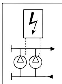
Each electric pump is controlled by a frequency converter. The starting priority is changed in accordance with the time set in the relevant parameter field on frequency converter. The speed adjustment will apply to all the electric pumps installed.
