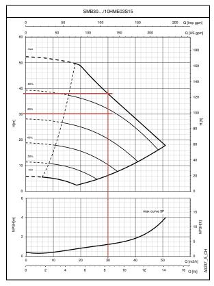
When selecting SMB booster sets, the performance levels of the pump must be taken into account.
