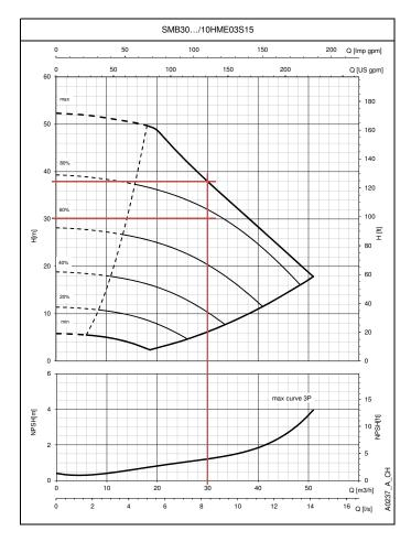
The example alongside refers to a required flow rate of 30 m<sup>3</sup>/h and a pressure of 30 m water column
