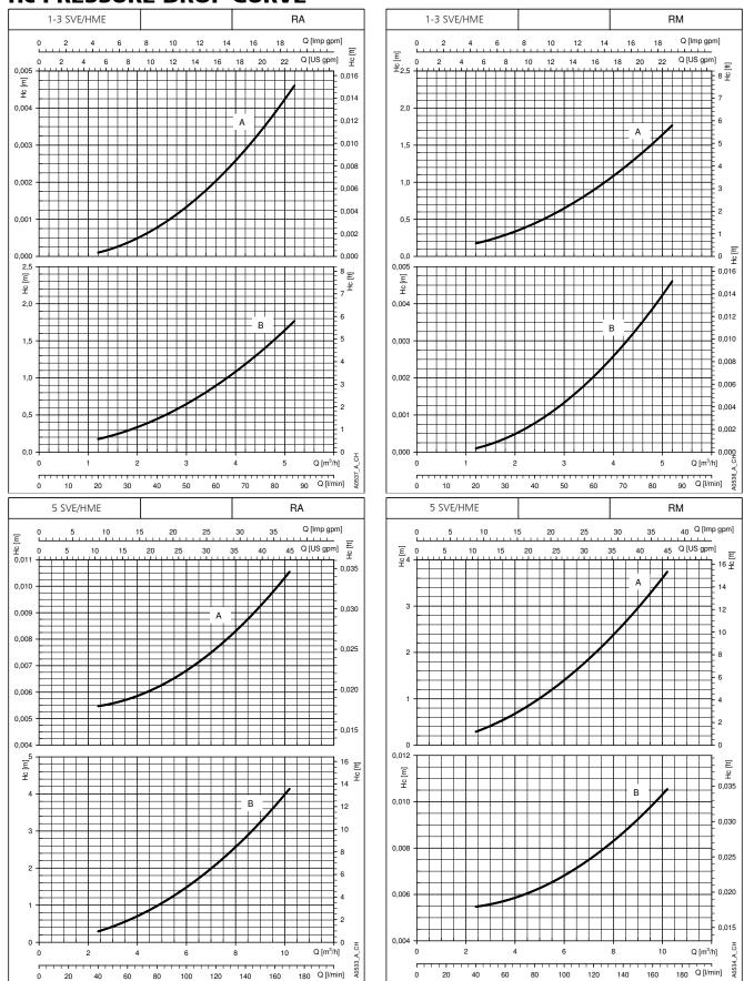
The declared curves are valid for liquids with density  $\rho=1$  Kg/dm³ and kinematic viscosity  $\nu=1$  mm²/sec.
