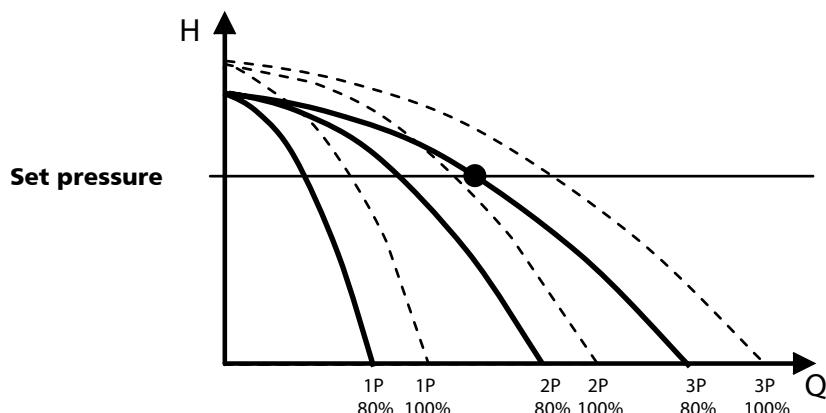
When the demand for water decreases, the electric pumps switch off in succession. The number of revolutions of the first electric pump switched on decreases to a set minimum before switching off.
