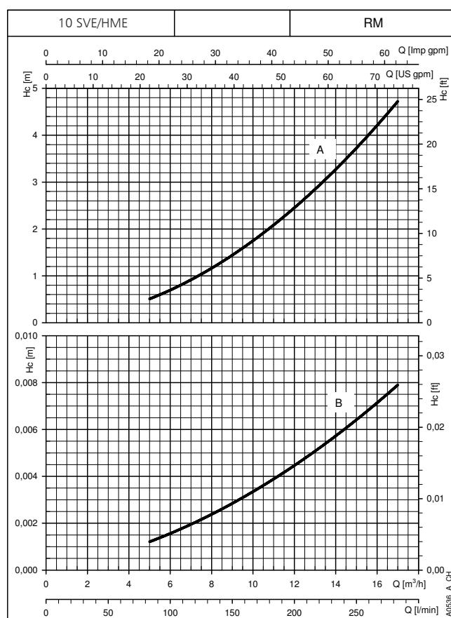
The declared curves are valid for liquids with density  $\rho = 1 \text{ Kg/dm}^3$  and kinematic viscosity  $\nu = 1 \text{ mm}^2/\text{sec}$ .
