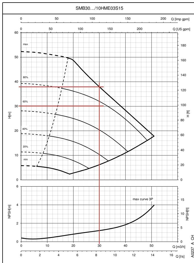
The example alongside refers to a required flow rate of  $30 \text{ m}^3/\text{h}$  and a pressure of  $30 \text{ m}$  water column
