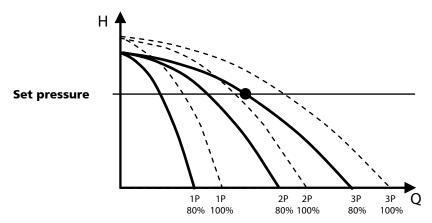
When the demand for water decreases, the electric pumps switch off in succession. The number of revolutions of the first electric pump switched on decreases to a set minimum before switching off.
