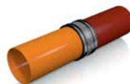
Center coupling over joint. Tighten clamps and shear band reciprocally.
