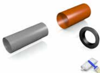
Position pipe ends.
