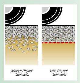
Without an effective geotextile, the aggregate base can break down and become mixed with water and soil creating mud - this reduces the shear strength and compaction of the aggregate. Woven geotextiles provide long-term separation by improving compaction and preventing the contamination of the aggregate. With such a comprehensive range Rhyno® can provide woven geotextiles to suit a wide variety of subgrades or soils.
