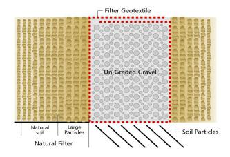
Wrapping less expensive ungraded gravels in woven geotextile allows water to pass through and acts as a barrier to soil particles. In this way, Rhyno® creates a natural filter adjacent to the geotextile, giving a more reliable filtration capability. Available in a wide range of pore sizes it can be matched with differing soil types for optimum performance.
