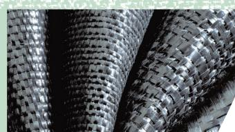
**Woven Polypropylene Geotextiles**
