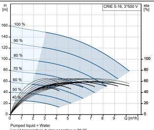
Pumped liquid = Water Liquid temperature during operation = 20  $^{\circ}$ C Density = 998.2 kg/m³
