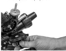
3. Remove the propeller from the housing to clear any debris that may be trapped inside.
