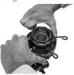
For 360° operation, remove both adjustment rings.
