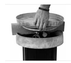
After all retaining segments have been positioned, recheck to make sure they are completely under the logo cap.
