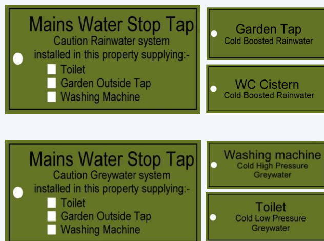
Figure 4: examples of labels for use at stop valve and other key connection points
